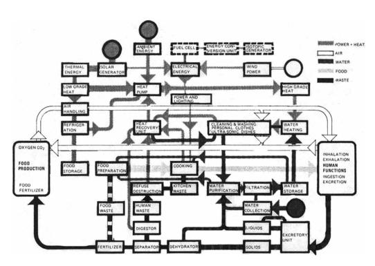
Figure 2. Alexander Pike's 'Basis diagram for a hypothetical autonomous servicing unit.' At Cambridge University he suggested ways to reorder buildings so that they would be as autonomous as cabin ecological systems and thus not harm the environment. Pike, 'Cambridge Studies', Architectural Design, 42 (July, 1972), p. 442.
